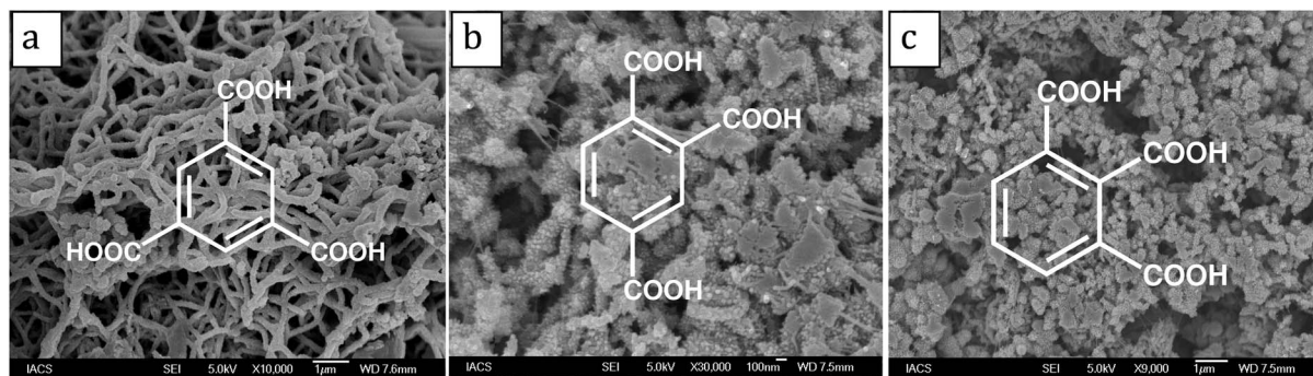
Fig. 1 FESEM-images of (a) BTA-1/PANI, (b) BTA-2/PANI and (c) BTA-3/PANI. Synthesis conditions: [acid]/[aniline] = 0.25, [aniline]/[APS] = 1.00.
